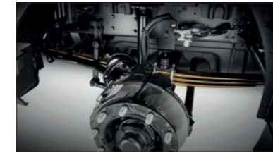
Long taper spring suspension
