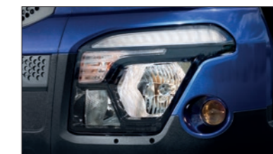
Headlamps / LED Daytime Running Lights The light distribution surfaces of the headlamps have been maximized to improve visibility at night and for added style and safety, LED DRLs have been applied.
